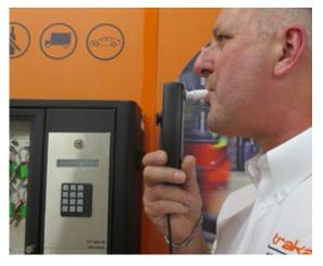
A five second blow and the system will confirm a Pass or a Fail. Only if Passed will the key be released. A Fail and the key will be locked in place. Furthermore, the Fail will be logged in the Traka database together with the user's name.
